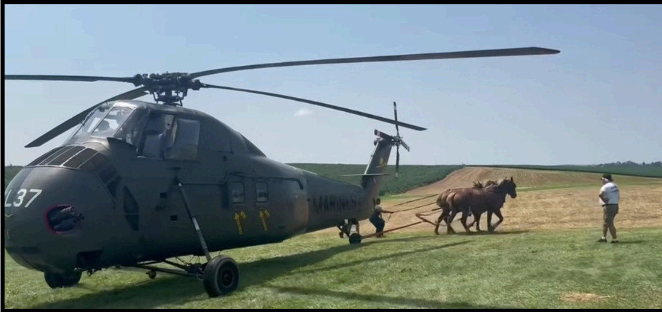
Jim Stuart and his Belgian mares Jinger and Paulee, pulling a Vietnam War-era helicopter at the Antique Power Show in Marshalltown. The helicopter needed its tail slightly uphill to start due to the fuel system being gravity fed.
